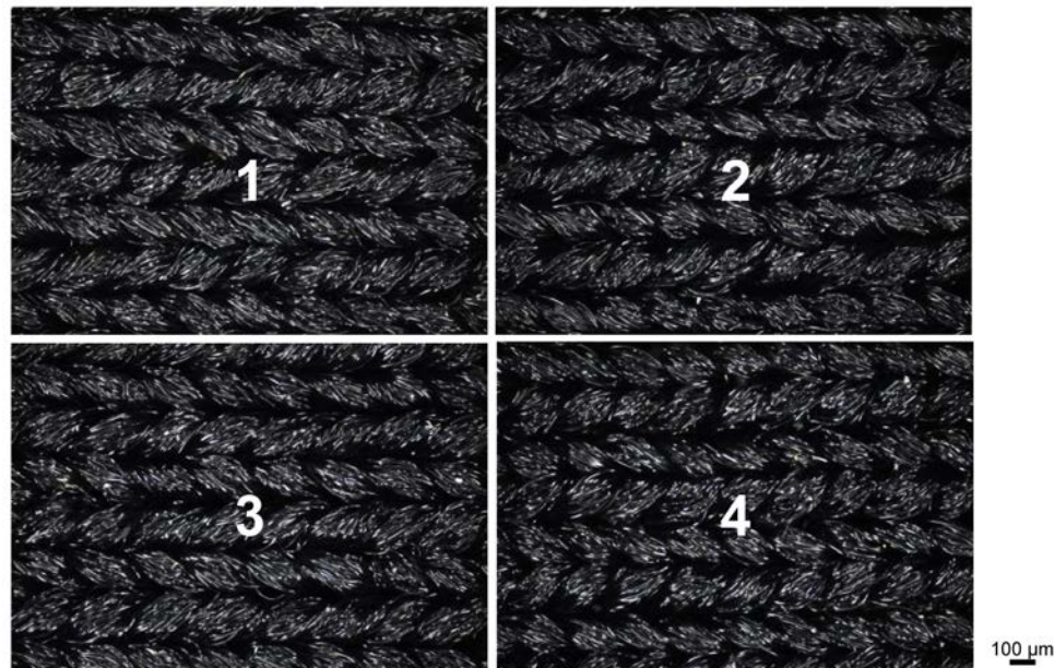
Fig. 1. Color optical microscope images of the fabric samples confirm that all samples have the same color and knit structure. Sample identifier numbers are overlaid in white.
